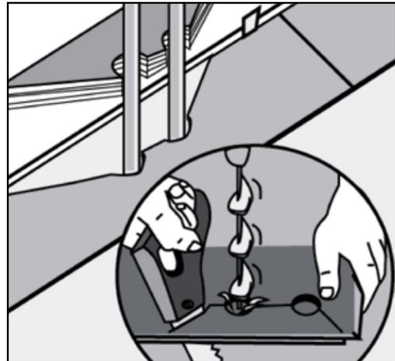
**8** Where there are pipes or other obstructions, drill holes in the planks that are 10mm bigger than the pipe diameter and then cut the piece to facilitate installation. Use matching pipe covers for a neat finish.
